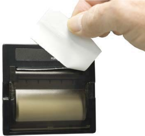
Figure 3-16 Trimming off Extra Paper
