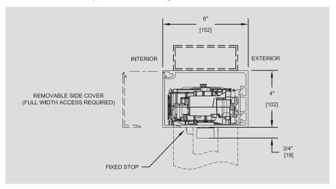
Elevation view Overhead concealed single operator center hung Right hand door shown (left hand opposite)
