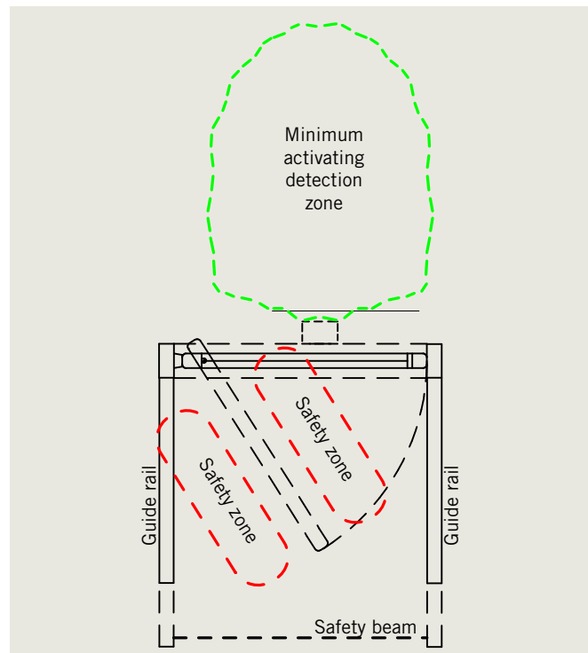
Fig. 5.1.2 One way traffic, door mounted presence sensors
